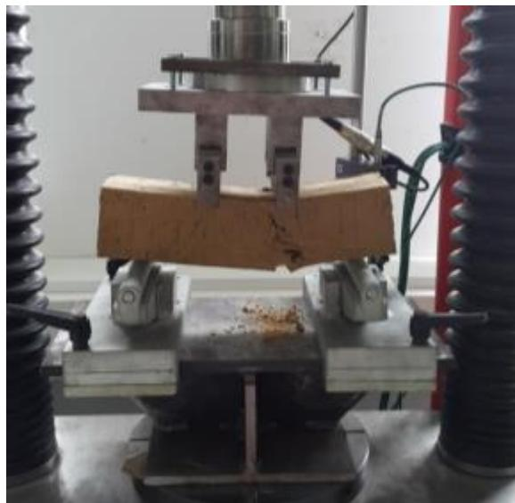
Four point bending strength test
