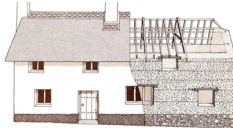
*A typical 17th century cob house showing some constructional details. The wall is built off a stone plinth in several layers, or lifts, and lintels and roof timbers are supported on the cob, using timber pads or cross pieces where necessary.*
