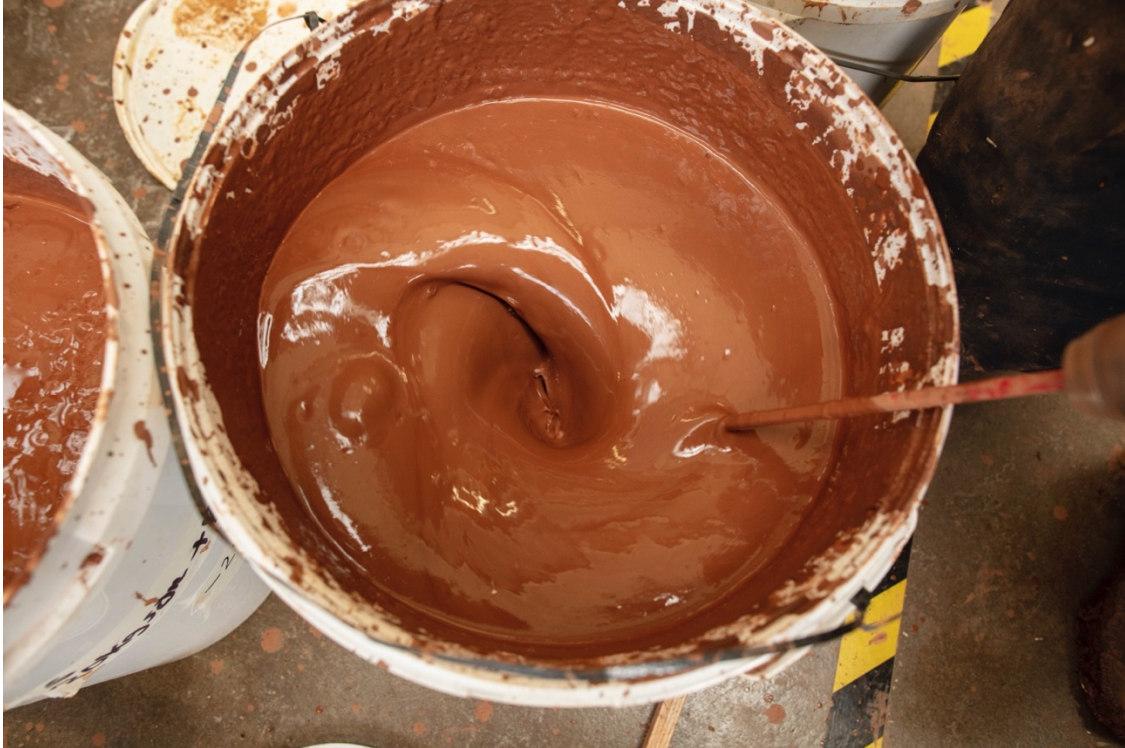
Figure 19. A photo showing the consistency of the earth slip. (Photo: Matthew Fox)
