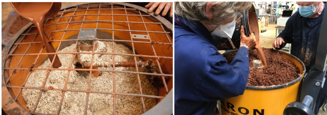
Figure 22. Photos showing the mixing of slip into hemp fibres. (Photo: Matthew Fox)
