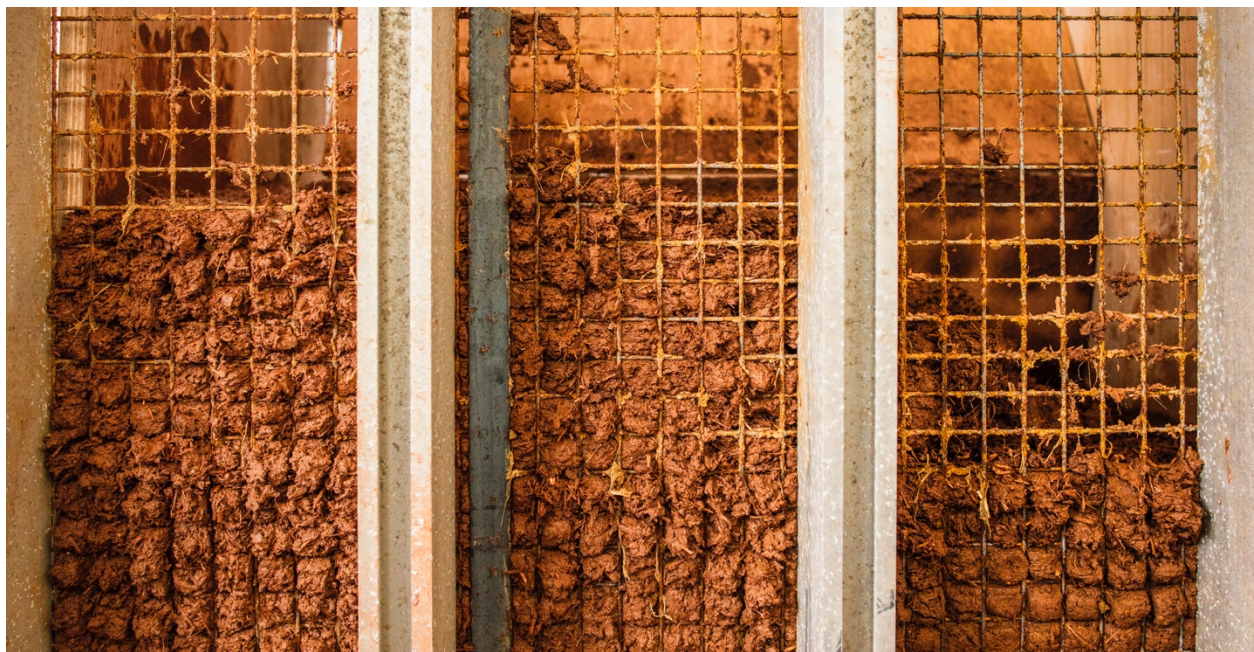
Figure 11. Photo showing thermal cob viewed through mesh. (Photo: Matthew Fox)
