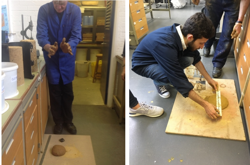
Figure 16. Photos of a drop ball test. (Photo: Matthew Fox)
