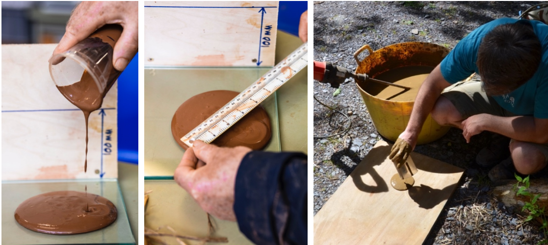
Figure 21. Photos of the puddle test. (Photo: Matthew Fox)
