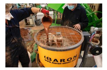
The clay rich slip is added to the hemp shiv in the mixer in a volumetric ratio of three parts shiv to one part slip. This represents a proportion of hemp shiv by 50% weight of dry soil.
